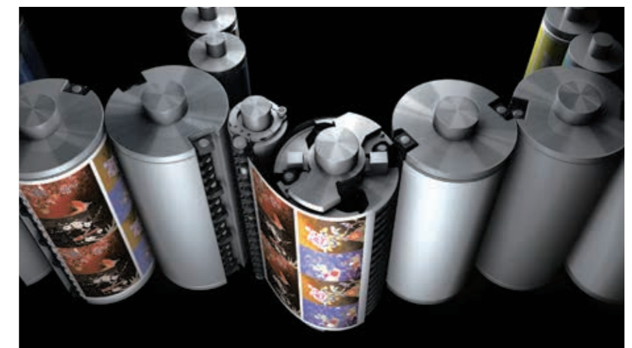
Double/double/single-diameter cylinder perfecting mechanism*
